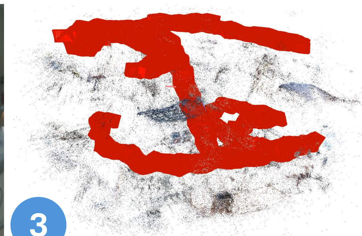
3 Determine the location of the camera in 3D using SfM (COLMAP); scale is arbitrary
