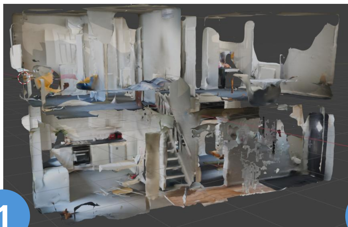
1 Create a LiDAR scan of the house using an iPad
